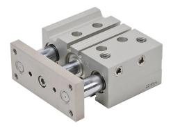
NITRA pneumatic cylinder, dual guide rod, 25mm bore, 12mm rod diameter, 25mm stroke, double acting, magnetic piston, universal mount.
