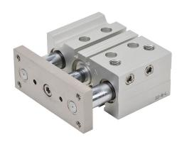
NITRA pneumatic cylinder, dual guide rod, 25mm bore, 12mm rod diameter, 20mm stroke, double acting, magnetic piston, universal mount.
