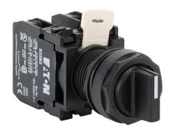
Eaton selector switch, 22mm, 3-position, spring return to center from right or left, (2) N.O. contact(s), plastic base, plastic bezel, Operator: black, knob, 30mm, round, plastic.
