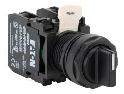
Eaton selector switch, 22mm, 3-position, spring return to center from right or left, (2) N.O. contact(s), plastic base, plastic bezel, Operator: black, knob, 30mm, round, plastic.
