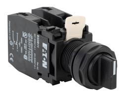
Eaton selector switch, 22mm, 3-position, maintained, (1) N.O./(1) N.C. contact(s), plastic base, plastic bezel, Operator: black, knob, 30mm, round, plastic.
