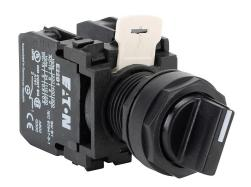
Eaton selector switch, 22mm, 2-position, maintained, (1) N.O./(1) N.C. contact(s), plastic base, plastic bezel, Operator: black, knob, 30mm, round, plastic.
