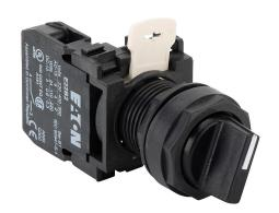
Eaton selector switch, 22mm, 2-position, maintained, (1) N.O. contact(s), plastic base, plastic bezel, Operator: black, knob, 30mm, round, plastic.
