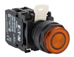
Eaton pushbutton, 22mm, momentary, incandescent illuminated, (1) N.O. contact(s), plastic base, plastic bezel, Operator: amber, extended, 28mm, round, plastic, 24 VAC/VDC, full voltage.
