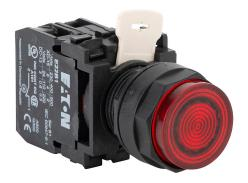
Eaton pushbutton, 22mm, momentary, incandescent illuminated, (1) N.C. contact(s), plastic base, plastic bezel, Operator: red, extended, 28mm, round, plastic, 24 VAC/VDC, full voltage.
