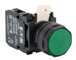
Eaton pushbutton, 22mm, momentary, (1) N.O. contact(s), plastic base, plastic bezel, Operator: green, flush, 28mm, round, plastic.
