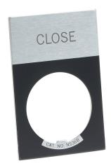
Eaton jumbo legend plate, aluminum, rectangular, black field, silver background, black engraved text, legend plate marking "CLOSE". For use with 22mm pilot devices.
