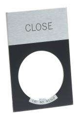
Eaton jumbo legend plate, aluminum, rectangular, black field, silver background, black engraved text, legend plate marking "CLOSE". For use with 22mm pilot devices.
