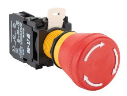
Eaton emergency stop pushbutton, 22mm, trigger action twist-to-release, (1) N.C. contact(s), plastic base, plastic bezel, Operator: red, mushroom, 40mm, round, plastic.
