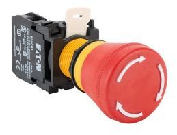
Eaton emergency stop pushbutton, 22mm, trigger action twist-to-release, (1) N.C. contact(s), plastic base, plastic bezel, Operator: red, mushroom, 40mm, round, plastic.
