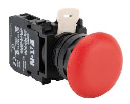
Eaton emergency stop pushbutton, 22mm, push to lock, pull to reset, (1) N.C. contact(s), plastic base, plastic bezel, Operator: red, mushroom, 40mm, round, plastic.
