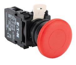
Eaton pushbutton, 22mm, momentary, (1) N.C. contact(s), plastic base, plastic bezel, Operator: red, mushroom, 40mm, round, plastic.
