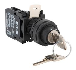
Eaton selector switch, 22mm, 2-position, spring return from right, key removable in all positions, (1) N.O. contact(s), plastic base, plastic bezel, Operator: black, key, 30mm, round, plastic.
