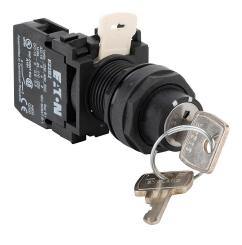
Eaton selector switch, 22mm, 2-position, maintained, key removable in all positions, (1) N.O. contact(s), plastic base, plastic bezel, Operator: black, key, 30mm, round, plastic.
