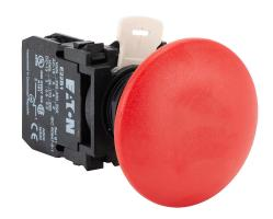
Eaton emergency stop pushbutton, 22mm, push to lock, pull to reset, (1) N.C. contact(s), plastic base, plastic bezel, Operator: red, mushroom, 50mm, round, plastic.
