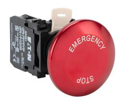
Eaton emergency stop pushbutton, 22mm, push to lock, pull to reset, (1) N.C. contact(s), plastic base, plastic bezel, Operator: red, mushroom, 50mm, round, aluminum, operator text "EMERGENCY STOP".
