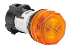
Eaton incandescent indicating light, permanent light function, 22mm, amber, 29mm, round, plastic base, 120 VAC/VDC, full voltage.
