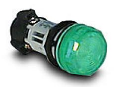
Eaton cluster style LED indicating light, permanent light function, 22mm, green, 29mm, round, plastic base, 120 VAC/VDC, full voltage.
