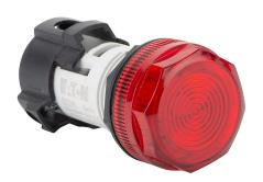
Eaton cluster style LED indicating light, permanent light function, 22mm, red, 29mm, round, plastic base, 120 VAC/VDC, full voltage.
