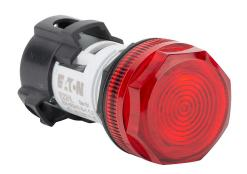
Eaton cluster style LED indicating light, permanent light function, 22mm, red, 29mm, round, plastic base, 24 VAC/VDC, full voltage.
