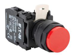
Eaton pushbutton, 22mm, momentary, (1) N.C. contact(s), plastic base, plastic bezel, Operator: red, extended, 28mm, round, plastic.
