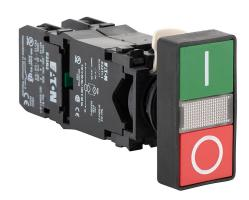
Eaton pushbutton, 22mm, momentary, incandescent illuminated, (1) N.O./(1) N.C. contact(s), plastic base, plastic bezel, Operator: red/green, double headed, 58mm, rectangular, plastic, operator text "(I) and (0)", 120 VAC, transformer.
