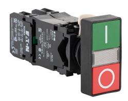
Eaton pushbutton, 22mm, momentary, incandescent illuminated, (1) N.O./(1) N.C. contact(s), plastic base, plastic bezel, Operator: red/green, double headed, 58mm, rectangular, plastic, operator text "(I) and (0)", 120 VAC, transformer.
