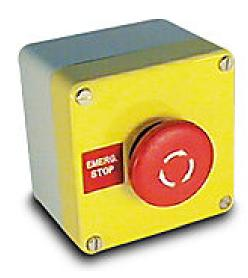
Eaton emergency stop control station, single pushbutton, mushroom, red, twist-to-release, (1) N.C. contact(s), legend plate marking "EMERG. STOP".
