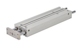
NITRA pneumatic cylinder, dual guide rod, 20mm bore, 10mm rod diameter, 250mm stroke, double acting, magnetic piston, universal mount.
