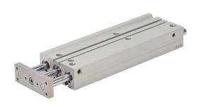
NITRA pneumatic cylinder, dual guide rod, 20mm bore, 10mm rod diameter, 200mm stroke, double acting, magnetic piston, universal mount.
