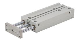
NITRA pneumatic cylinder, dual guide rod, 20mm bore, 10mm rod diameter, 150mm stroke, double acting, magnetic piston, universal mount.
