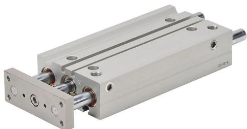
NITRA pneumatic cylinder, dual guide rod, 20mm bore, 10mm rod diameter, 125mm stroke, double acting, magnetic piston, universal mount.
