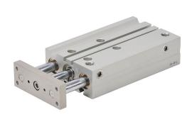
NITRA pneumatic cylinder, dual guide rod, 20mm bore, 10mm rod diameter, 100mm stroke, double acting, magnetic piston, universal mount.
