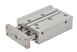
NITRA pneumatic cylinder, dual guide rod, 20mm bore, 10mm rod diameter, 75mm stroke, double acting, magnetic piston, universal mount.
