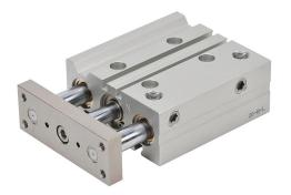
NITRA pneumatic cylinder, dual guide rod, 20mm bore, 10mm rod diameter, 50mm stroke, double acting, magnetic piston, universal mount.
