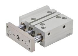
NITRA pneumatic cylinder, dual guide rod, 20mm bore, 10mm rod diameter, 40mm stroke, double acting, magnetic piston, universal mount.
