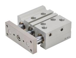
NITRA pneumatic cylinder, dual guide rod, 20mm bore, 10mm rod diameter, 25mm stroke, double acting, magnetic piston, universal mount.
