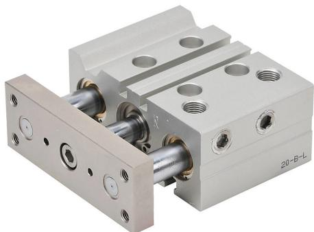
NITRA pneumatic cylinder, dual guide rod, 20mm bore, 10mm rod diameter, 20mm stroke, double acting, magnetic piston, universal mount.
