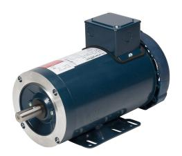
Marathon XRI premium efficiency AC induction motor, inverter rated, 2hp, 3-phase, 208-230/460 VAC, 1800rpm, TEFC, NEMA 145TC frame, rolled steel, C-face/rigid base mount.
