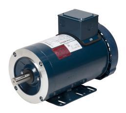
Marathon XRI premium efficiency AC induction motor, inverter rated, 1-1/2hp, 3-phase, 208-230/460 VAC, 1800rpm, TEFC, 145TC frame, rolled steel, C-face/rigid base mount.
