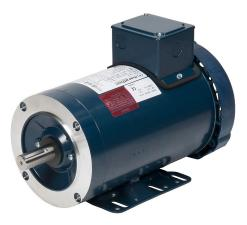
Marathon XRI premium efficiency AC induction motor, inverter rated, 1-1/2hp, 3-phase, 208-230/460 VAC, 1800rpm, TEFC, NEMA 145TC frame, rolled steel, C-face/rigid base mount.
