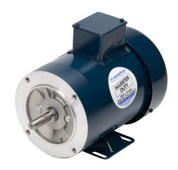
Marathon XRI premium efficiency AC induction motor, inverter rated, 1hp, 3-phase, 208-230/460 VAC, 3600rpm, TEFC, 56C frame, rolled steel, C-face/rigid base mount.
