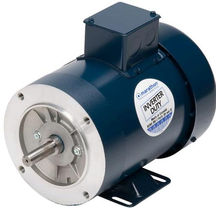
Marathon XRI premium efficiency AC induction motor, inverter rated, 1hp, 3-phase, 208-230/460 VAC, 3600rpm, TEFC, NEMA 56C frame, rolled steel, C-face/rigid base mount.
