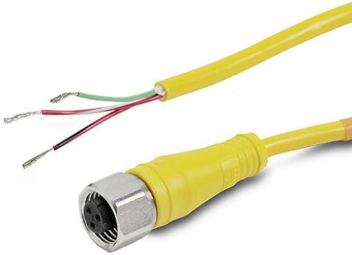
AutomationDirect connection cable, 1/2in-20 UNF thread axial female to pigtail, 3-pole, PVC jacket, yellow, 32.8ft/10m cable length, IP67 IP68 IP69K.
