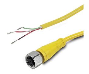
AutomationDirect connection cable, 1/2in-20 UNF thread axial female to pigtail, 3-pole, PVC jacket, yellow, 16.4ft/5m cable length, IP67 IP68 IP69K.
