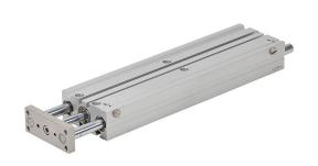
NITRA pneumatic cylinder, dual guide rod, 16mm bore, 8mm rod diameter, 200mm stroke, double acting, magnetic piston, universal mount.
