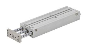
NITRA pneumatic cylinder, dual guide rod, 16mm bore, 8mm rod diameter, 175mm stroke, double acting, magnetic piston, universal mount.
