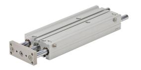
NITRA pneumatic cylinder, dual guide rod, 16mm bore, 8mm rod diameter, 150mm stroke, double acting, magnetic piston, universal mount.
