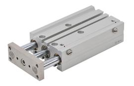
NITRA pneumatic cylinder, dual guide rod, 16mm bore, 8mm rod diameter, 75mm stroke, double acting, magnetic piston, universal mount.
