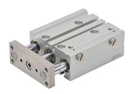
NITRA pneumatic cylinder, dual guide rod, 16mm bore, 8mm rod diameter, 40mm stroke, double acting, magnetic piston, universal mount.
