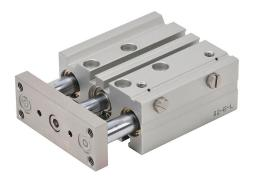
NITRA pneumatic cylinder, dual guide rod, 16mm bore, 8mm rod diameter, 30mm stroke, double acting, magnetic piston, universal mount.
