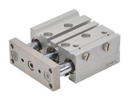
NITRA pneumatic cylinder, dual guide rod, 16mm bore, 8mm rod diameter, 20mm stroke, double acting, magnetic piston, universal mount.
