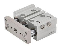
NITRA pneumatic cylinder, dual guide rod, 16mm bore, 8mm rod diameter, 10mm stroke, double acting, magnetic piston, universal mount.
