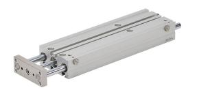
NITRA pneumatic cylinder, dual guide rod, 12mm bore, 6mm rod diameter, 150mm stroke, double acting, magnetic piston, universal mount.
