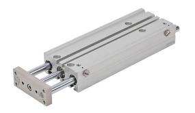
NITRA pneumatic cylinder, dual guide rod, 12mm bore, 6mm rod diameter, 125mm stroke, double acting, magnetic piston, universal mount.
