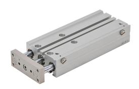
NITRA pneumatic cylinder, dual guide rod, 12mm bore, 6mm rod diameter, 100mm stroke, double acting, magnetic piston, universal mount.
